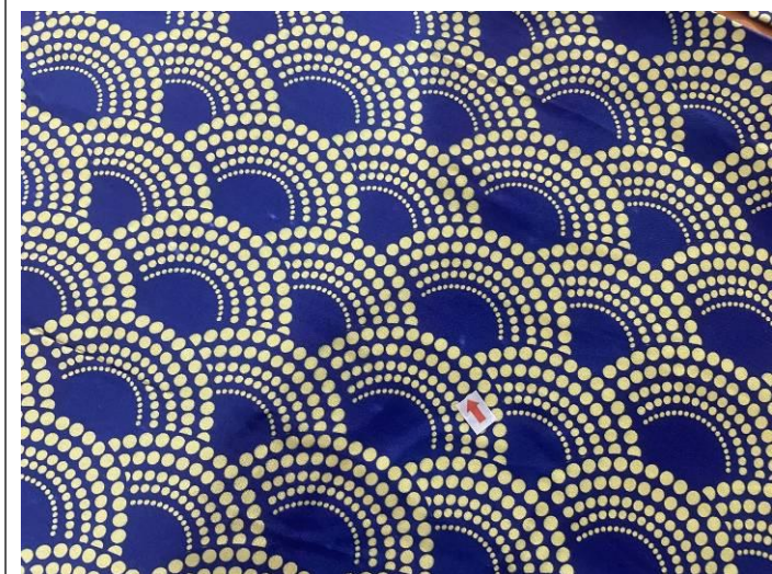
Leaky white- -Major
